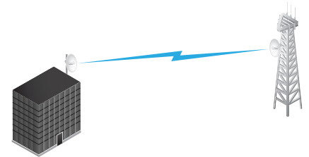
Dish Reflector Design Use a NanoBeam on each side of a PtP link.
