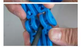
The Jonard Tools **patented** and **award-winning** FOD-2000 Fiber Optic Drop Cable Slitter simplifies the slitting of drop cable jackets at mid span or end sections and is perfect for FTTH technicians working with flat fiber drop cables. This drop cable slitter features the following:
