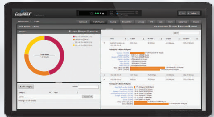
The Traffic Analysis screen displays status information about the traffic traveling through the EdgeRouter, including the local hosts and types of network traffic.
