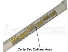
copper hard-line provides a low loss path to the antenna's central splitting and phasing component. The brass radiating elements of the HG2409U-PRO utilize an air dielectric for lowest loss and superior radiating efficiency. The design is factory tuned for superior performance.
