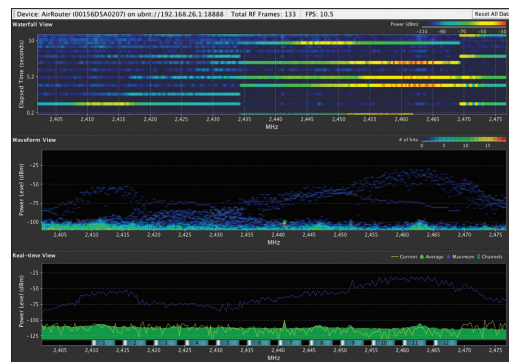
AirView Tool provides real-time wireless signal statistics
